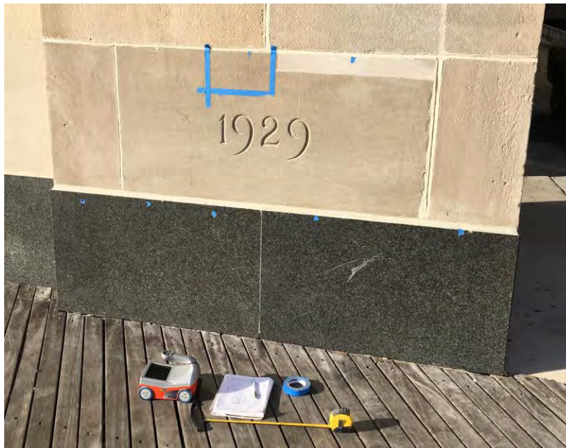
Fig 5: NDE equipment identified embedded metal box thought to be a time capsule in the corner stone
